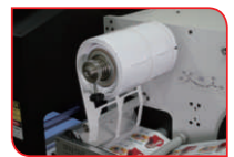
Matrix removal Scrap papers can be easily removed.
