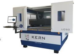
it the fastest and most productive laser system in their product lineup. An improved down draft vacuum table is built into the system ensuring consistent fume removal and material hold down over the entire table top.
